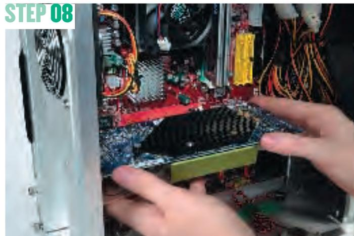
**FIT GRAPHICS CARD** Like most other 5900/5950 cards, our GeForce uses two PCI slots because it runs hot enough that a big heatsink and fan is required to keep it cool. Using the extra slot isn't a problem – our motherboard has so much built-in that we have no shortage of PCI slots. It does need a dedicated power supply from the PSU to get anything beyond VESA graphics though.
