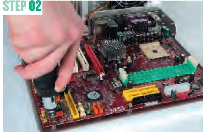
**ATTACH THE MAINBOARD** Wearing your anti-static wristband, screw the motherboard onto the chassis backplane. You'll usually need to put spacers into the board first and screw the motherboard onto them. The more screws you can use, the better – some cards need substantial pressure to fit. NOTE: the Athlon 64 CPU requires a heatsink backplate attached to the rear of the motherboard.
