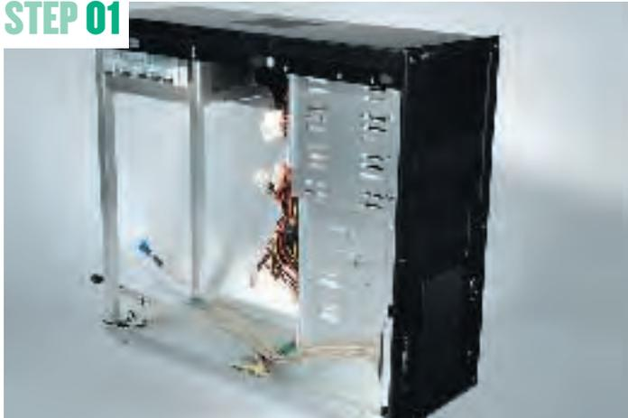
**STRIP THE CASE** In order to get started fitting the core components of the machine, you need to take both sides off the case, remove the chassis backplane, and untie all the wires. The Praetorian box has a handy caddie for the backplane and thumbscrews where possible, which makes all this quite easy, and screwdriver-free too.
