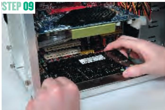
**SLOT IN SOUND CARD** Pick a free PCI slot and use it for the sound card. NOTE that we put our sound card pretty much as far away from the graphics card as it could go, to give the GeForce card as much room to cool as it can. As there are quite a few wires to connect into the card if you want to (such as the optical drive), you might want to leave it at least one up from the bottom for easy access.
