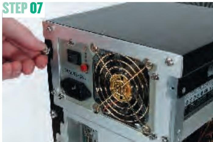
**SCREW SIDE PANEL ON** Again, as we had significant amounts of dust in our fitting environment, we decided to put the left-hand case panel on to keep the motherboard protected – unless you're super-scrupulous about cleaning your office/workplace, you should consider this too. We'll be removing the left-hand panel briefly later on to screw in drives.
