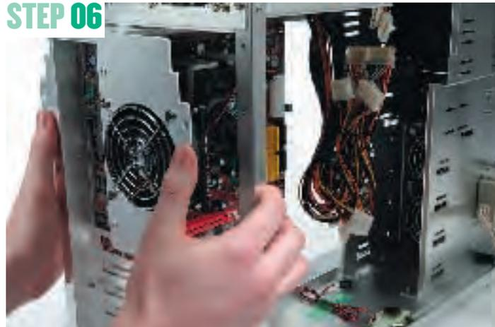
**REPLACE THE BACKPLANE CHASSIS** With the CPU and heatsink fitted, it's now time to re-insert the backplane chassis so that we can start putting the rest of the components in. As experienced case-modders and PC builders will know, you can – technically – do a lot more with the chassis out, but our fitting environment was far from dust-free, so it's just not worth the risk.
