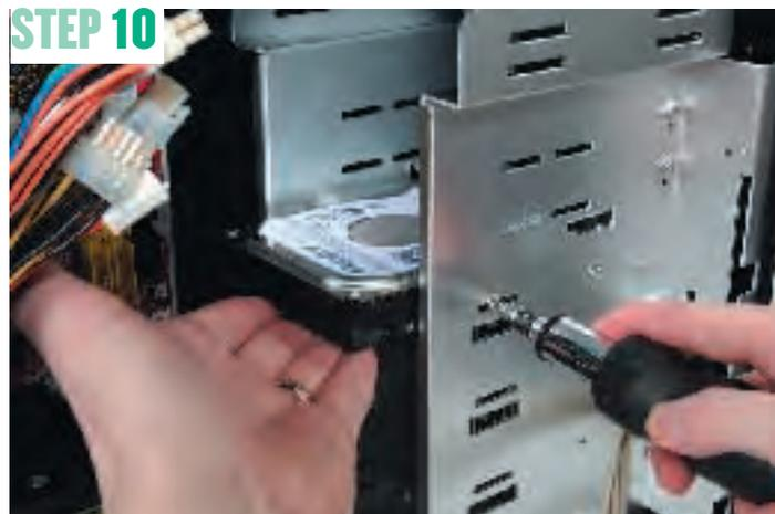
**ATTACH HARD DRIVES** Our Ultimate Linux box boasts two hard drives, and we fitted them quite low in the chassis. The reason for this is because the Cooler Master case that we chose has fans specifically for the hard drives, and we wanted them to get maximum usage. The drives were connected up to the Promise SATA RAID controller for maximum performance.
