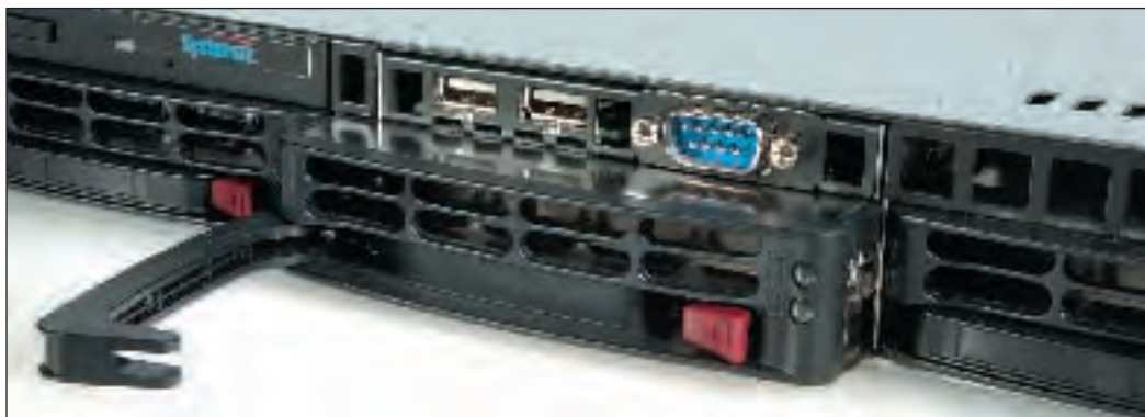
Four drive bays, but only two hard drives – that's one way of keeping costs down! There's no PS/2 port either...
